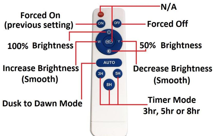
For first use, press the “AUTO” button on the [solar light control panel](#) to activate the light and remote.
